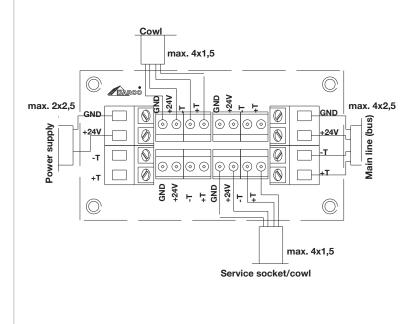
Side power connection with main line (bus) cable size higher than 4x1,5 (connection inside the junction box)
